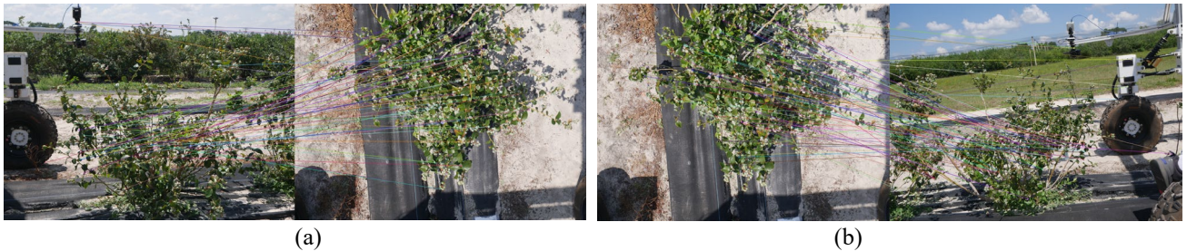
Figure 6. Illustration of image matching with Oriented FAST and Rotated Brief (ORB) algorithm. Actually, there are many mismatching pairs of features points obviously. For example, the feature points on the robot mistakenly match to the points of blueberry plant. (a) matching result between right view and top view; (b) matching result between top view and left view.
