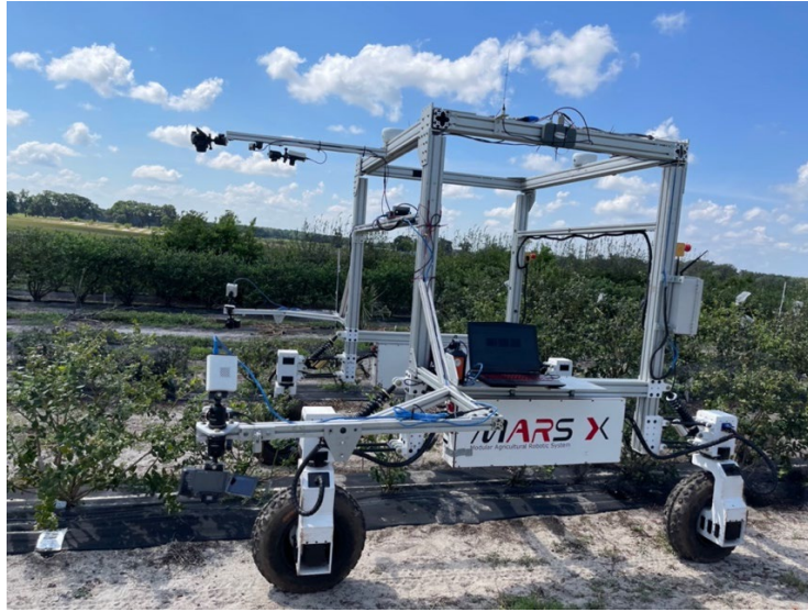
Figure 2. Multi-view imaging system is integrated with a ground robotic platform. The imaging system possesses three different types of camera system (RGB, RGB-GPS, RGBD-GPS) and 9 cameras in total. Each camera system can capture the blueberry image from top, left-side and right-side to minimize the occlusion by leaves and trunks.
